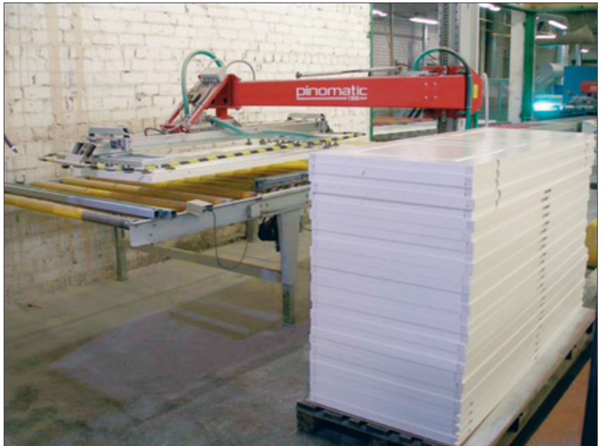
Pinomatic 1900 stacker at the end of finishing line.
