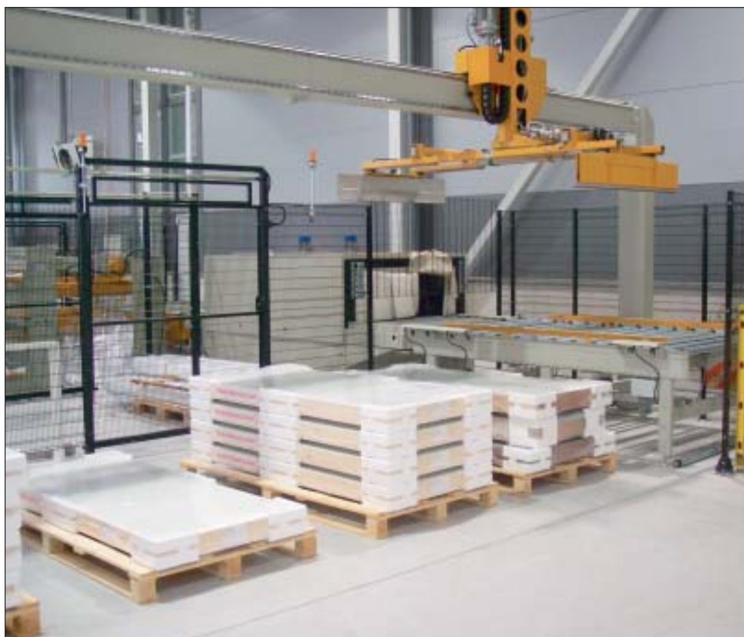
A Pinomatic 2405 stacker at the end of the line stacks prepared packages onto pallets for individual orders.
