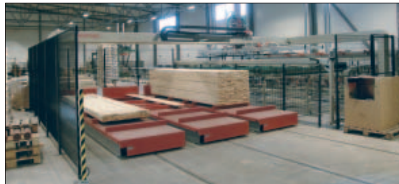
Three different lengths of timber can be used simultaneously, with own stacking stations on carriages that move aside.
