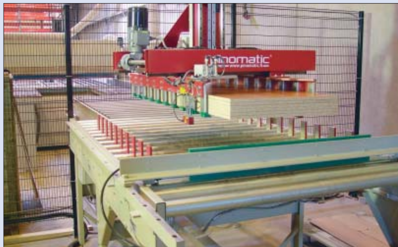
Lifting of heavy board bundles is now possible with the new Pinomatic stacker.
